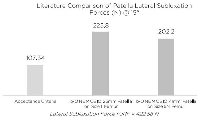
Figure 3. The resistance of the MOBIO™ TKA patellar component to frank subluxation is nearly double anticipated physiologic loads at 15 degrees of flexion. This was true for all combinations tested.
