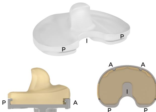
**Figure 7.** The locking mechanism of the MOBIO™ (b-ONE) knee. The mechanism engages posteriorly (P) with locking tabs which resists liftoff in hyperextension. Anteriorly (A), a CoCr wire on the insert engages with two metal barbs on the tray. There is also a press fit of the insert along the island (I) located anterior to the PCL cutout on the tray. These three locking strategies (A, P and I) engage to secure the insert in the sagittal and coronal planes to minimize micromotion.
