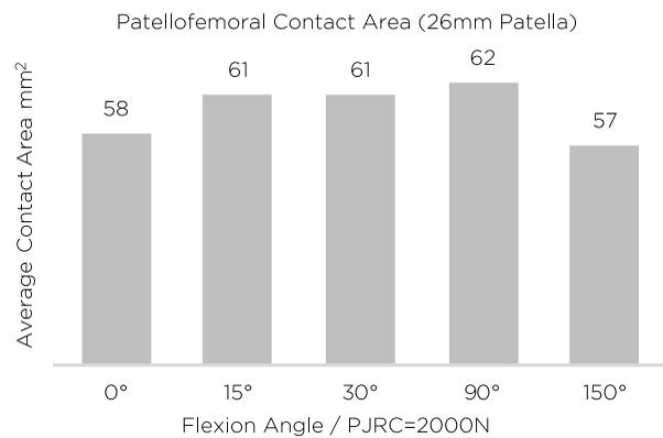
Figure 7: Patella contact area increases with the flexion angle from 0° to 90° of flexion, thus reducing the contact stress.
