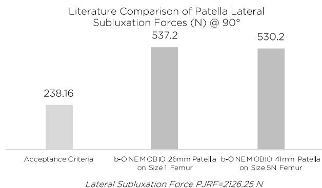
Figure 5. At 90 degrees of flexion the forces required to sublux the MOBIO™ patella were significantly higher than the patella is expected to experience anatomically. This was true for all configurations tested. This suggests that the MOBIO™ design would effectively resist lateral subluxation of the patella.
