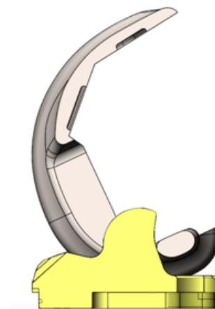
Figure 3. By designing the cam post contact point to be more distal on the tibial post, the jump height is larger which provides additional security against subluxation.
