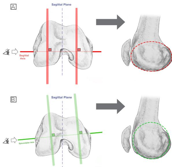
**Figure 4 A&B.** Figure A shows the distal end of the femur. The red line shows the sagittal plane from the MR theory. If the knee is viewed from the side along this J curve axis, the knee has an elliptical shape. In contrast, Figure B shows the SR axis which is coincident with the epicondylar axis. When the knee is viewed down this axis, the profile is circular. This circular profile of the SR knee design is indicated when the femoral bone is resected in external rotation.
