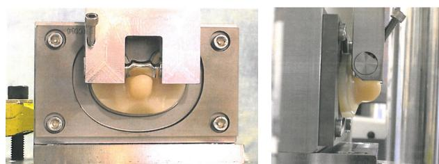
**Figure 6.** The fatigue loading setup for the MOBIO™ (b-ONE) PS knee. The cam cyclically loaded the post at a load that was three times anticipated physiological loading for ten million cycles.
