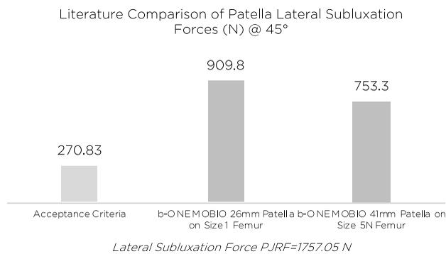
Figure 4. At 45 degrees of flexion, the MOBIO™ TKA patella offered significant resistance to lateral subluxation. The MOBIO™'s resistance to subluxation was much more than twice the levels anticipated in the patellofemoral joint.
